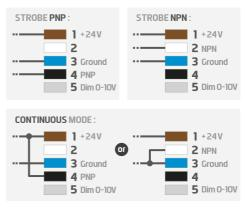
PNP: from 5 to 24V for 100% ON. From 0 to 1V for 100% OFF. NPN: less than 1V for 100% ON. Above 2V for 100% OFF. Max 20V.
