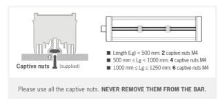
During the set up, the light has to be switched off and unplugged. Please use M4 screws and insert them in the captive nuts located in the back of the light. The light will be better fixed if you spread the attachment points symmetrically along the bar.
